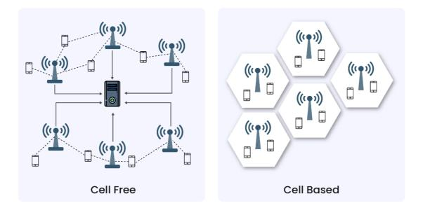
In this design the user is allowed to attach to multiple Base stations which coordinate among themselves to serve a user. Base Stations use their local Channel State Information (CSI) to compute the channel conditions rather than a shared global channel condition.
