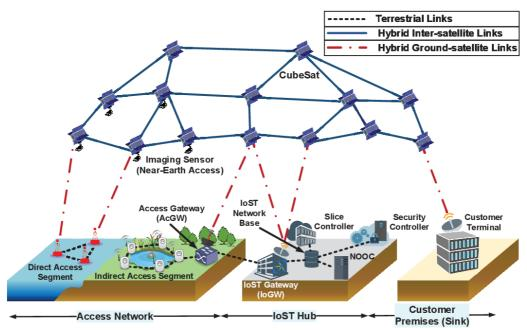
The physical architecture of IoST consists of the IoST Hubs, on-Earth and near-Earth sensing devices, and the CubeSat network. The IoST Hubs communicate with the CubeSats and house a large portion of control framework for the entire network, whereas the CubeSats operate in the exosphere (altitudes of 500 km and above) forming the network in space to receive, transmit, and relay data efficiently.
